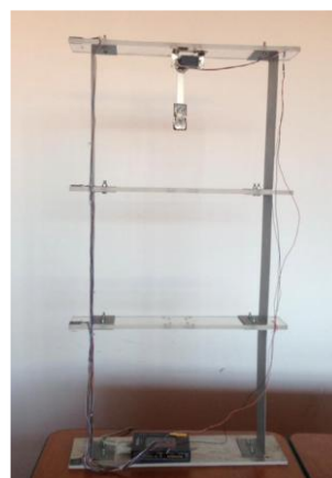
Stand experimental - Experimental three floor building for active vibration suppression
